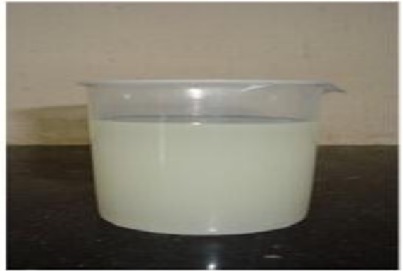
Glycerin is obtained after washing the oil with water
