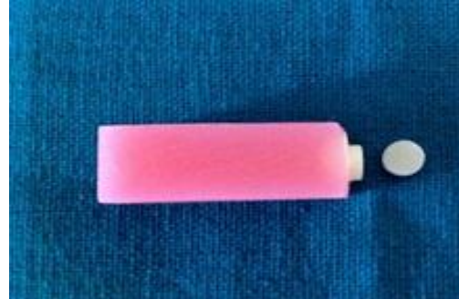
Figure 8. Fracture at the interface of composite resin and acrylic resin denture teeth.
