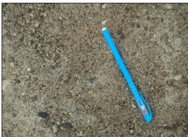
Figure 3. Finer bed load sample collected from middle reach of Panchanoi river bed
